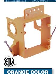
easily identifies low voltage application. EZLV2-NWN EZ BOX is a 2-gang, new work, low voltage bracket used for low voltage installations for new construction projects (new work) applications. The backless design is great for the large or deep low-voltage wiring needed for communications and cable installations, and it fits standard 2-gang faceplates. Round concentric knockouts allow for multiple fitting sizes.
