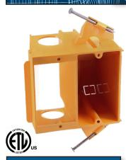
**ORANGE COLOR** easily identifies low voltage application. EDV2B EZ BOX is a 2-gang, new work, dual voltage bracket used in construction (new work) applications where dual-voltage applications need to be side by side. The backless design is great for the large or deep low-voltage wiring needed for communications and cable installations, and it fits standard 2-gang faceplates. Four knockouts and two round openings for EZ installation.
